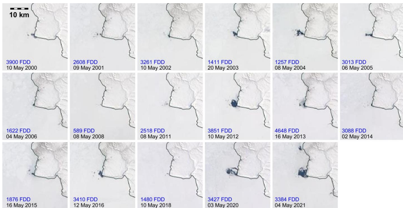
Figure 2: The presence of sensible heat polynya at Cape Jackson during winters when ice bridge in Nares Strait formed between 2000 and 2021 in MODIS imagery. Blue numbers correspond to the sum of freezing degree days (FDD) from a corresponding date of bridge formation (see Kirillov et al., 2021) to 30 April. Each panel is 37.5 x 37.5 km.
