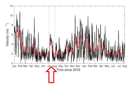
The wind velocity variation at Tehuantepec Gulf is shown in black. A moving average with 7-day interval is shown in red.
