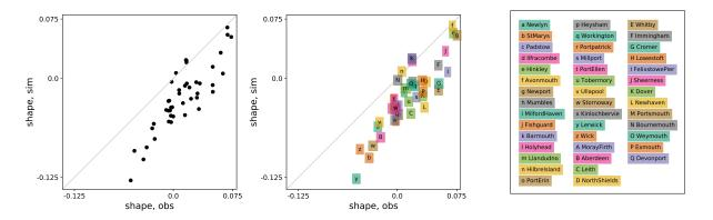
**Figure 1.** Left panel: Illustrating correlation between shape parameter as diagnosed from tide-gauge data (X-axis) and from a simulation (Y-axis), for sites on the UK coast. Pearson's R coefficient is 0.86. (The right and centre panels are shown to enable identification of some of the sites.)
