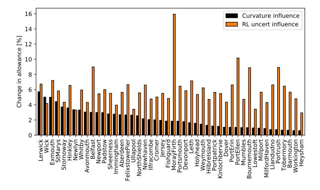
**Figure 4.** Following Howard and Palmer (2020), we show the sensitivity (black filled bars) of Hunter's allowance to curvature of the return level plot of still water level (in other words, sensitivity to the departure of the still water extremes from a Gumbel distribution). Also shown for comparison is the sensitivity to uncertainty in the return level curve. For full details of the method see Howard and Palmer (2020). Sites are ordered by curvature sensitivity (not geographical location).
