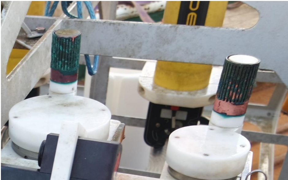
Figure R2: Filter and pump intake for the two CONTROS sensors from O246 directly after retrieval.
