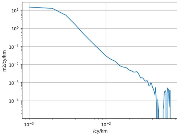
**Figure 2 : power spectral density (in  $\text{cm}^2/\text{cy}/\text{km}$ ) at  $60^\circ\text{W}$ ,  $35^\circ\text{N}$  from the along-track sea level anomalies of AltiKa satellite**
