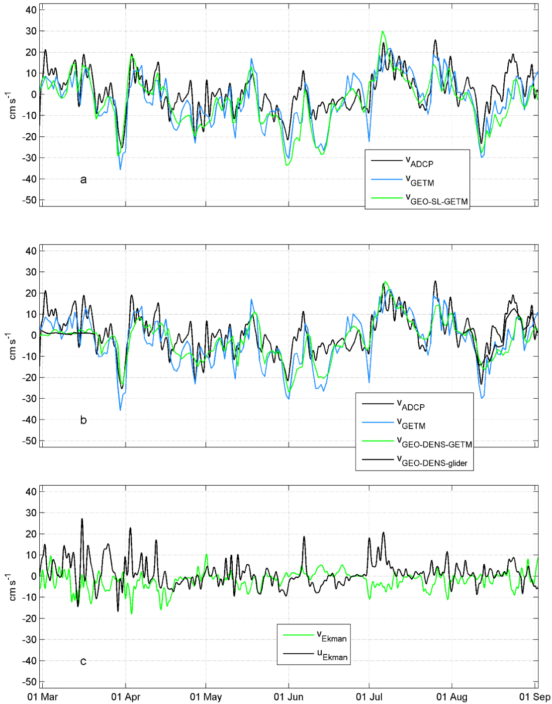
381 382 Figure 5. Temporal courses of (a and b) current velocity v -component (positive northward) measured by ADCP 383 ( V_{\text{ADCP}} ), simulated v -component ( V_{\text{GETM}} ), estimated from the GETM sea level data ( V_{\text{GEO-SL-GETM}} ), estimated 384 from temperature and salinity data collected by glider ( V_{\text{GEO-DENS-glider}} ), estimated from temperature and salinity 385 data simulated by GETM at 11 m depth ( V_{\text{GEO-DENS-GETM}} ). Mean Ekman current u -component (positive eastward) 386 and v -component ( U_{\text{Ekman}} and V_{\text{Ekman}} ) in the depth range 0–11 m (c). Time-series are shown from March to 387 September 2020 at the ADCP location (see Fig. 1b and c).
