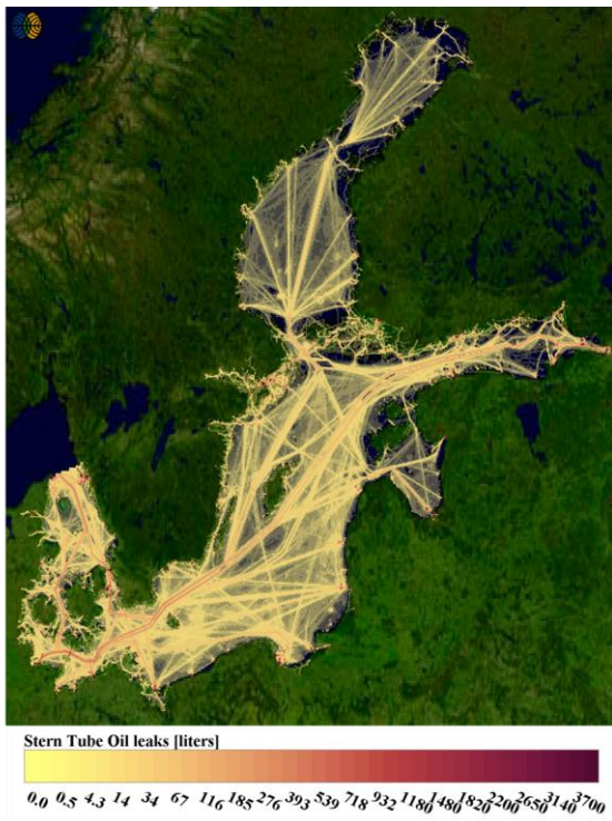
Figure 4 Distribution of the annual stern tube oil releases for year 2012 from the Baltic Sea shipping. Discharge volumes are indicated in liters per map grid area of 5 km 2 . Top right: Share of stern tube oil released in various sub-basins of the Baltic Sea (INL=Inland areas, RIG=Gulf of Riga, BOT=Bothnian Bay and Bothnian Sea, FIN=Gulf of Finland, KAT=Kattegat, BSP=Baltic Sea Proper). Lower bar chart depicts the monthly variation of stern tube oil discharges. Upper pie chart summarizes the contribution of various ship types to stern tube oil releases and the lower pie chart the flag state shares of stern tube oil releases. Map background Landsat-8 image courtesy of the U.S. Geological Survey.
