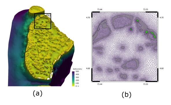
**Figure 3.** (a) Bathymetry of North Male' and Gaafaru atoll interpolated onto a simulation mesh. Bathymetry is exaggerated in the vertical for better visualisation, and shows that the individual complex features of the atoll are well captured. (b) Part of the unstructured mesh used for the simulations conducted in this work, focused on northern North Male' atoll. Mesh resolution is increased significantly at lagoons and coastlines.
