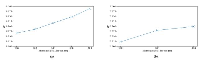
Figure 4. (a) Correlation between bathymetry interpolated onto mesh and the original high-resolution bathymetry dataset for different element sizes at lagoons. (b) Correlation between simulated tidal amplitudes and corresponding tide gauge data for the meshes identified in (a) that achieved  $R^2 > 0.9$ .
