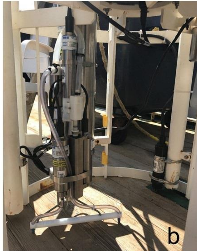
Fig. A1. SBE911 CTD-pump in- and outlet modification following the findings in van Haren and Laan (2016). (a) The T- and C-sensors clamped together with a structure holding in- and outlet pump-tubing of exactly the same diameter, separated at 0.3 m distance in the horizontal plane. (b) The modification of a. mounted in the CTD-frame.
