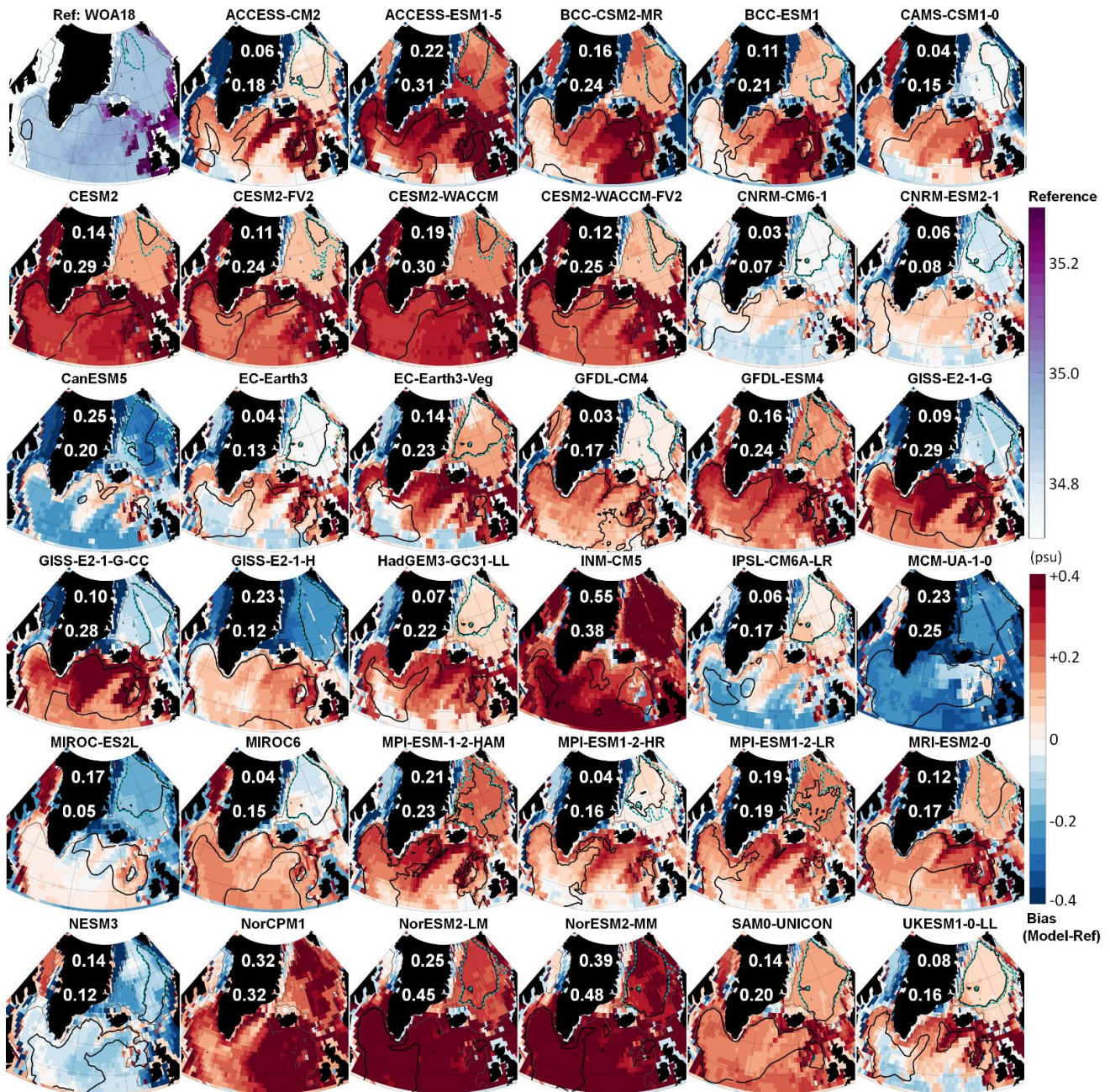
Figure A4. North Atlantic reference bottom practical salinity (top left panel, top colorbar), and for each CMIP6 model, bottom practical salinity bias (model minus reference) averaged over 1985-2014. White numbers for each model is its RMSE over the GIN (top) and SPG (bottom) areas, for depths over 1000 m. Thick black line indicates maximum mixed layer deeper than 1000 m; cyan dotted line in GIN, deeper than 700 m. Thin grey line, the 1000 m isobath.
