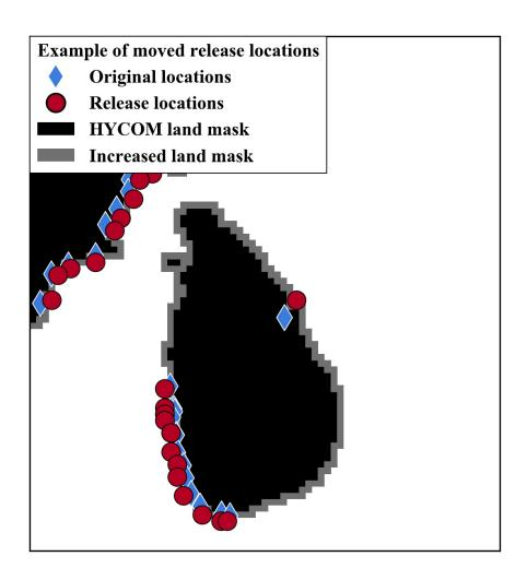
**Figure A2.** Example of original river source locations estimated by Lebreton et al. (2017) and moved release locations in relation to the HYCOM land mask around Sri Lanka. Release locations are shifted compared to original source locations where necessary to prevent particles from being released on or too close to land in particle tracking simulations.
