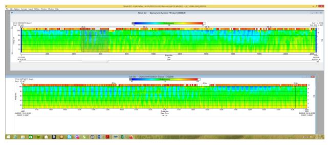
Figure shows acoustic backscatter data from a 300 kHz upward-looking Workhorse Sentinel ADCP by RDI deployed at CA13
