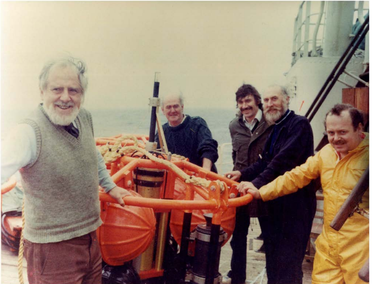
Figure 3. David Cartwright, FRS (1926-2015) (left) and colleagues around a 'Mark IV' bottom pressure recorder deployed to measure the tide in over 3000 m of water NE of the Azores in 1980. Others appearing the photograph (left to right): Ken Parry, Ian Vassie, Bev Hughes and Bob Spencer. Photograph courtesy of the National Oceanography Centre.
