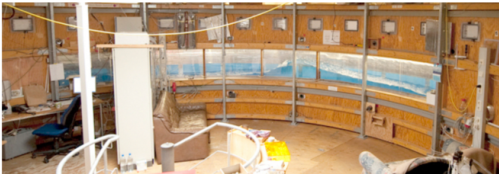
Figure 3: Heidelberg Aeolotron: Due to the infinite fetch of the 10 m diameter facility, long and steep breaking wind waves can be generated, much larger than in any linear facility.
