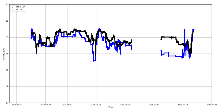
Fig. 4. The time series of TSG-measured salinity (black line) and collocated SMOS SSS measurements.
