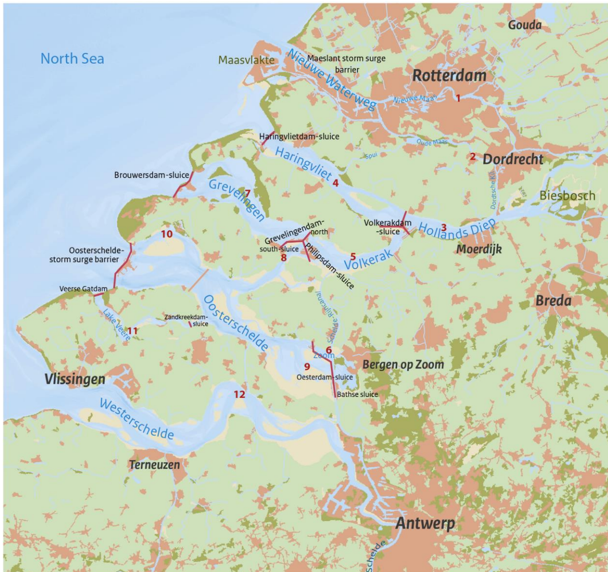
Figure R5: The Southwest Delta (Netherlands) with the main water basins and the main hydraulic infrastructures related to the Delta Works. Numbers indicate locations 1) Brienoord, 2) Puttershoek, 3) Bovensluis, 4) Haringvliet center, 5) Steenberg, 6) Zoom center, 7) Dreischor, 8) Zijpe, 9) Lodijkse Gat, 10) Hammen Oost, 11) Soelekerkepolder, 12) Hansweert. Source: Ysebaert et al., 2016.
