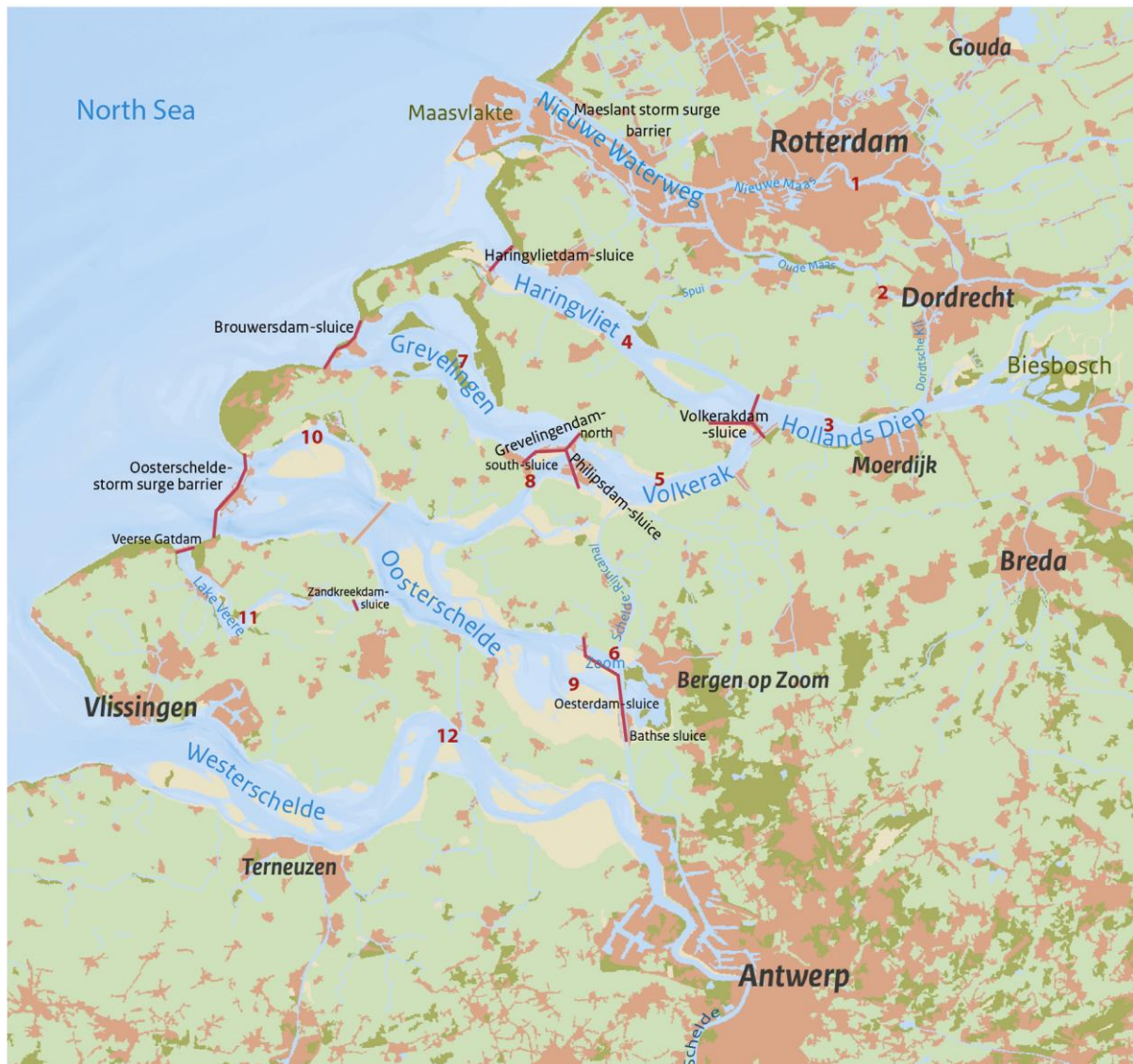
Figure R10: The Southwest Delta (Netherlands) with the main water basins and the main hydraulic infrastructures related to the Delta Works. Numbers indicate locations 1) Brienenoord, 2) Puttershoek, 3) Bovensluis, 4) Haringvliet center, 5) Steenberg, 6) Zoom center, 7) Dreischor, 8) Zijpe, 9) Lodijkse Gat, 10) Hammen Oost, 11) Soelekerkepolder, 12) Hansweert. Source: Ysebaert et al., 2016.
