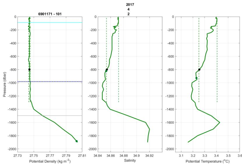
Figure R2. Same than Fig. R2 but for profile 6901171 – 101. Additionally, the horizontal lines on the left side plot represent the MLDs estimated by the Holte and Talley’s method: in gray the MLD defined by the density threshold, in black the MLD defined by the density algorithm, in blue the MLD defined by the temperature threshold and in cyan the MLD defined by the temperature algorithm; note that black and blue lines are overlapping.
