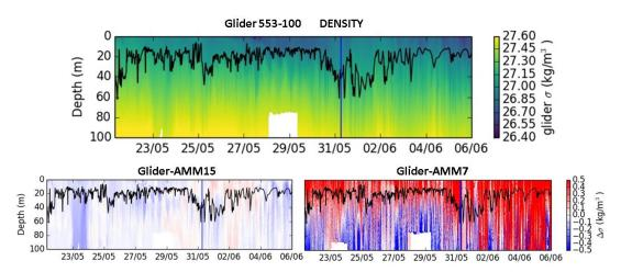
Figure 15: Top 100m density profile along glider 553-100 trajectory. Top panel: salinity measured by the Glider. Bottom left: difference glider-AMM15. Bottom right: difference glider-AMM7. The vertical blue line represents when the glider goes over the shelf break, crossing the 200m isobath. Before that time the glider is on the shelf. The black line is the MLD computed from the glider measurements.
