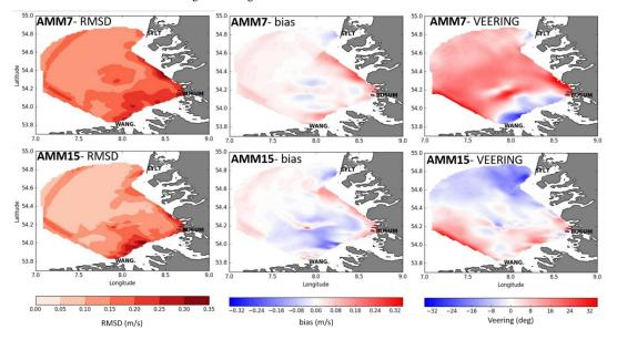
Figure 6: plots of statistics between HF radar surface current observations and AMM7 (top) and AMM15 (bottom) for the high-5 passed filtered data (tidal signal). Bias (observation-model) and RMSD (in m/s) are estimated on the velocity vector magnitudes. Right panel: phase or veering. Positive (negative) veering represent a clockwise (counter-clockwise) angle of AMM7 (top) or AMM15(bottom) vectors with respect to the HF radar vectors.
