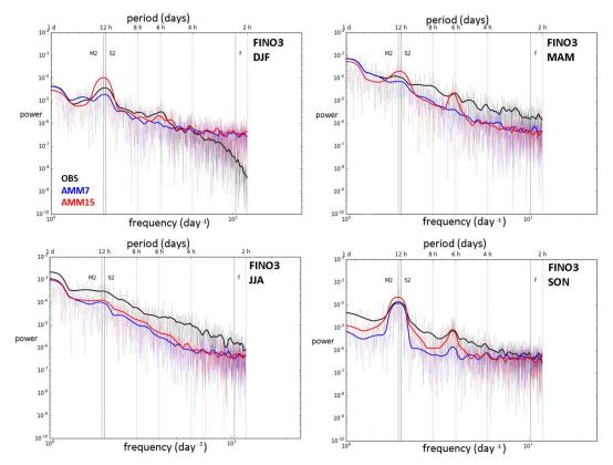
Figure 9: Power spectrum of SST for the FINO3 buoy (black line) compared with the AMM7 (blue) and AMM15 (red) simulations for December 2016 to February 2017 (top left), March to May 2017 (top right), June to August 2017 (bottom left) and September to November 2017 (bottom right).
