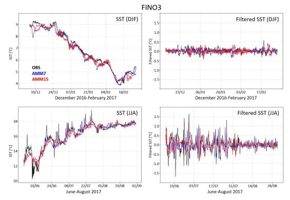
Figure 8: Timeseries of sea surface temperature (left) and filtered SST (right) for the FINO 3 buoy for December 2016-February 2017 (top) and June-August 2017 (bottom). Observations are shown in black, AMM7 in blue and AMM15 in red.
