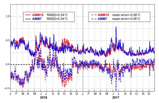
Figure 7: OSTIA minus Model SST RMSD and bias daily comparison for AMM7 (blue) and AMM15 (red) for the whole domain (negative mean error indicates a warm model bias).
