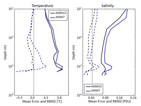
5 Figure 10: Observation minus model temperature (left) and salinity (right) profile assessment for AMM15 (black) and AMM7 (blue) for the whole domain. The RMS difference is shown by the solid lines and mean error (observation-model) is shown by the dashed lines.
