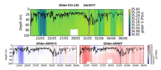
Figure 14: Top 100m of salinity profile along glider 553-100 trajectory. Top panel: salinity measured by the Glider. Bottom left: difference glider-AMM15. Bottom right: difference glider-AMM7. The vertical blue line represents when the glider goes over the shelf break, crossing the 200m isobath. Before that time the glider is on the shelf. The black line is the MLD computed from the glider measurements.
