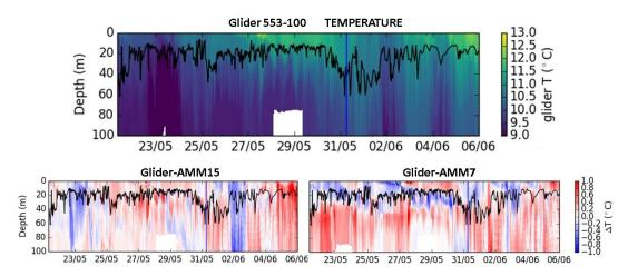
Figure 13: Top 100m of temperature profile along glider 553-100 trajectory. Top panel: temperature measured by the Glider. Bottom left: difference glider-AMM15. Bottom right: difference glider-AMM7. The vertical blue line represents when the glider goes over the shelf break, crossing the 200m isobath. Before that time the glider is on the shelf. The black line is the MLD computed from the glider measurements.
