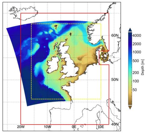
Figure 1: EMODnet bathymetry, in meters (logarithmic scale), showing the AMM15 model domain. The red line defines the AMM7 model domain. The yellow dotted box is the domain covered by the AMM15 products delivered on a regular grid to the Copernicus users. Figure modified from Graham et al. (2018). The bathymetry colour range has logarithmic scale.
