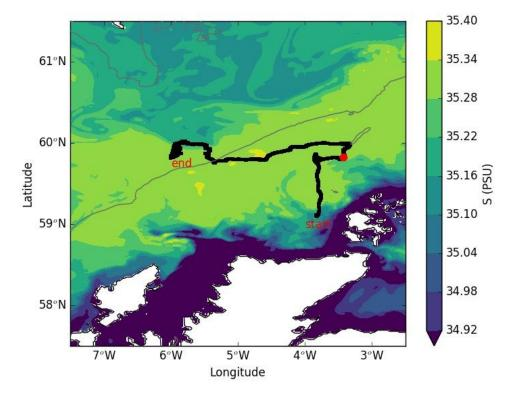
15 Figure 12: Glider 553 trajectory. The glider started the measurement close to the Scotland coast, and then moved towards the shelf break. The black line is the glider trajectory. The grey line represents the 200m isobath. The red dot is the glider position on the 23rt May 2017. The field on the background in the salinity on the 23<sup>rd</sup> of May.
