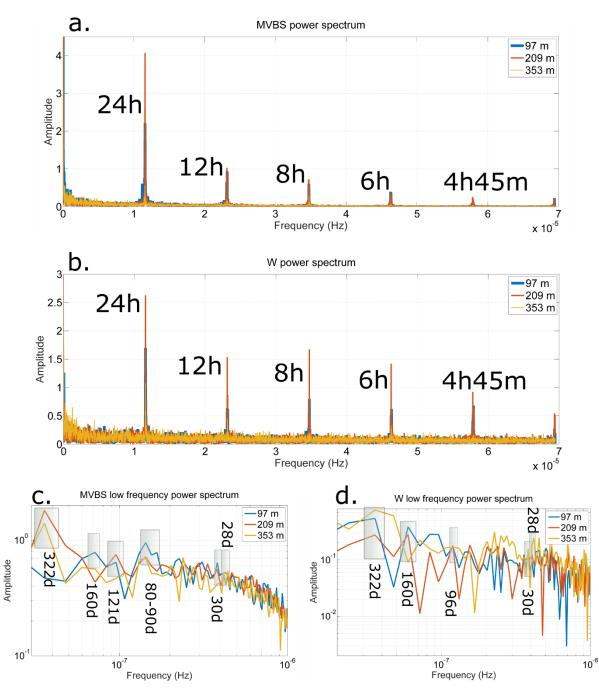
Figure 5: (a) Power spectrum of MVBS (high frequency range) at three selected bins (97m, 209m, 353m); (b) same as (a) but for W; (c) power spectrum of the low-passed MVBS time series (low frequency range) at three selected bins (97m, 209m, 353m); (d) same as (b) but for W.
