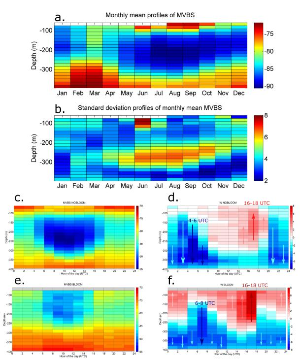
Figure 4: Monthly mean (a) vertical MVBS profiles and their standard deviation (b); (c-d) mean MVBS and W during non-blooming periods (approximately between May and November) as a function of depth and of the hour of the day; (e-f) mean MVBS and W during blooming periods (approximately between December and April) as a function of depth and of the hour of the day. Bluish and reddish arrows in (d) and (f) indicate main downward and upward motions, respectively.
