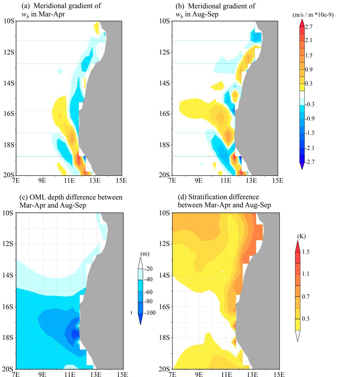
**Figure S1.** Meridional gradient of the vertical motion at the bottom of OML for (a) March-April mean and (b) August-September means. (c) Difference in OML depth ( $D$  in Eq. 3.5) between March-April and August-September mean. (d) Difference in upper ocean stratification ( $\Delta\theta$  in Eq 3.5) between March-April and August-September mean.
