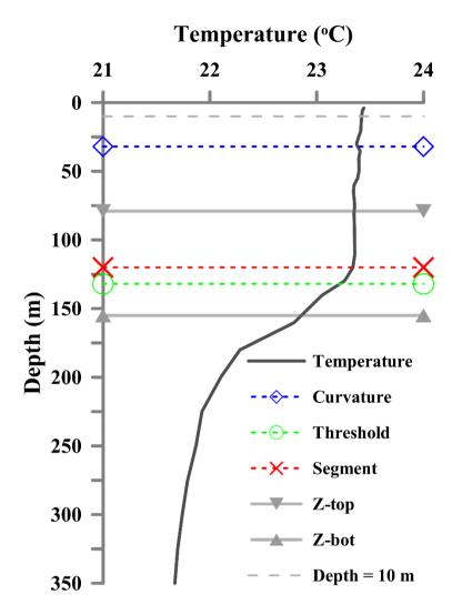
**Figure.** The MLD estimated for a schematic temperature profile based on curvature, threshold, and segment methods. Z-top and Z-bot represents the top and bottom ends of the portion of the profile with significant inhomogeneity.
