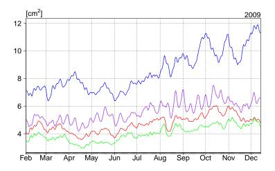
**Figure 4.** Temporal evolution of the SSH error variance in the ocean analysis over the period February-December 2009. Results obtained comparing the SSH of the ocean analysis in the experiments OSSE1 (blue lines) and OSSE2 (purple line), OSSE3 (red line) and OSSE4 (green line) with the data of the NR considering the ocean areas with a bathymetry deeper than 200 metres; y-axes expressed as  $[cm^2]$ . OSSE0 (not shown) ranged between 25 and 35  $cm^2$ .
