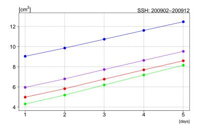
**Figure 5.** Variance of the error for each day of forecast (5 days) considering the SSH, in regions with a bathymetry deeper than 200 metres, over the period from Frebruary to December 2009. The legend of the OSSEs is as in Figure 4; y-axes expressed as  $[cm^2]$ .
