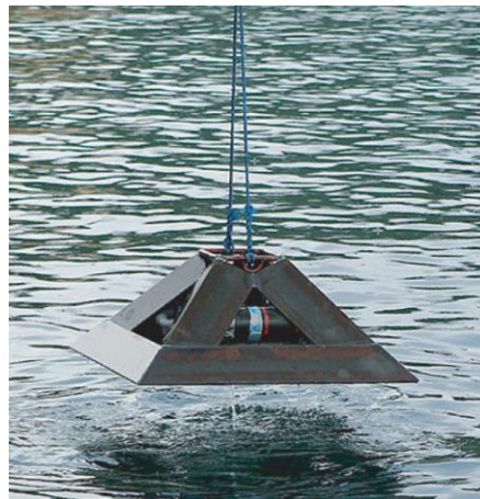
Figure S1. Left panel: An ADCP in a trawl-proof frame (yellow) onboard a research vessel, ready for deployment. Right panel: A bottom temperature logger (BTL) including temperature sensor, acoustic modem, and batteries in a trawl-proof frame.
