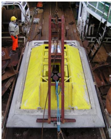
Figure S1. Left panel: An ADCP in a trawl-proof frame (yellow) onboard a research vessel, ready for deployment. Right panel: A bottom temperature logger (BTL) including temperature sensor, acoustic modem, and batteries in a trawl-proof frame.
