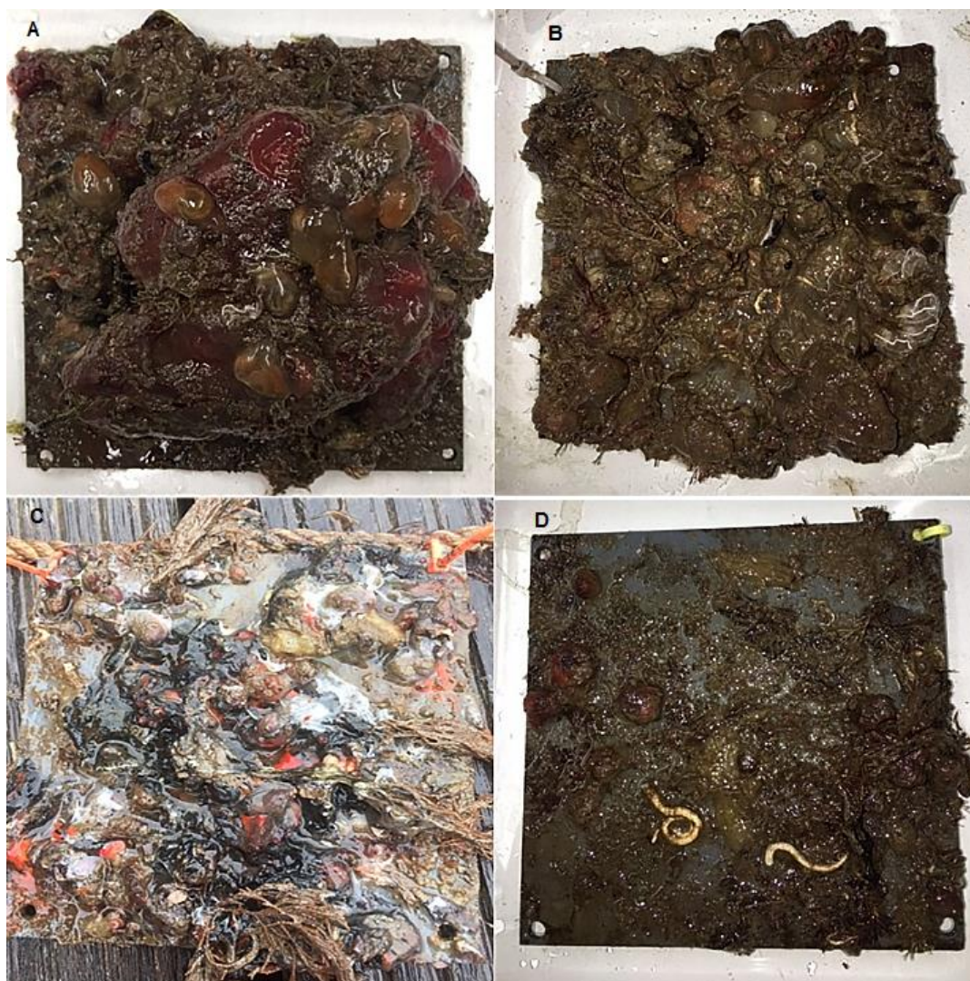
Figure 2. A) Settlement panel one week after exposure to a 33 psu treatment showing the high biomass and diverse biofouling community that had developed over two years at 1.5 m depth in a marina off Plymouth, UK. B) Example of a panel one week after exposure to a 20 psu treatment with many members of the biofouling community still alive. C) Panel one week after a 7 psu treatment showing black sulphurous rotting tissues. D) Typical panel appearance one month after exposure to 7 psu showing a much reduced fouling community.
