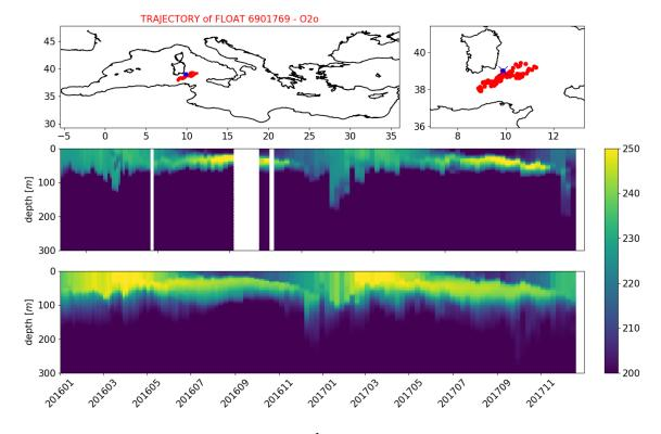
Figure 11: Hovmoller diagrams of oxygen concentration (mmol/m³) of one selected BGC-Argo float 6901769 (top panels) and model outputs (bottom panels) matched-up with float position for the period 2016-2017.
