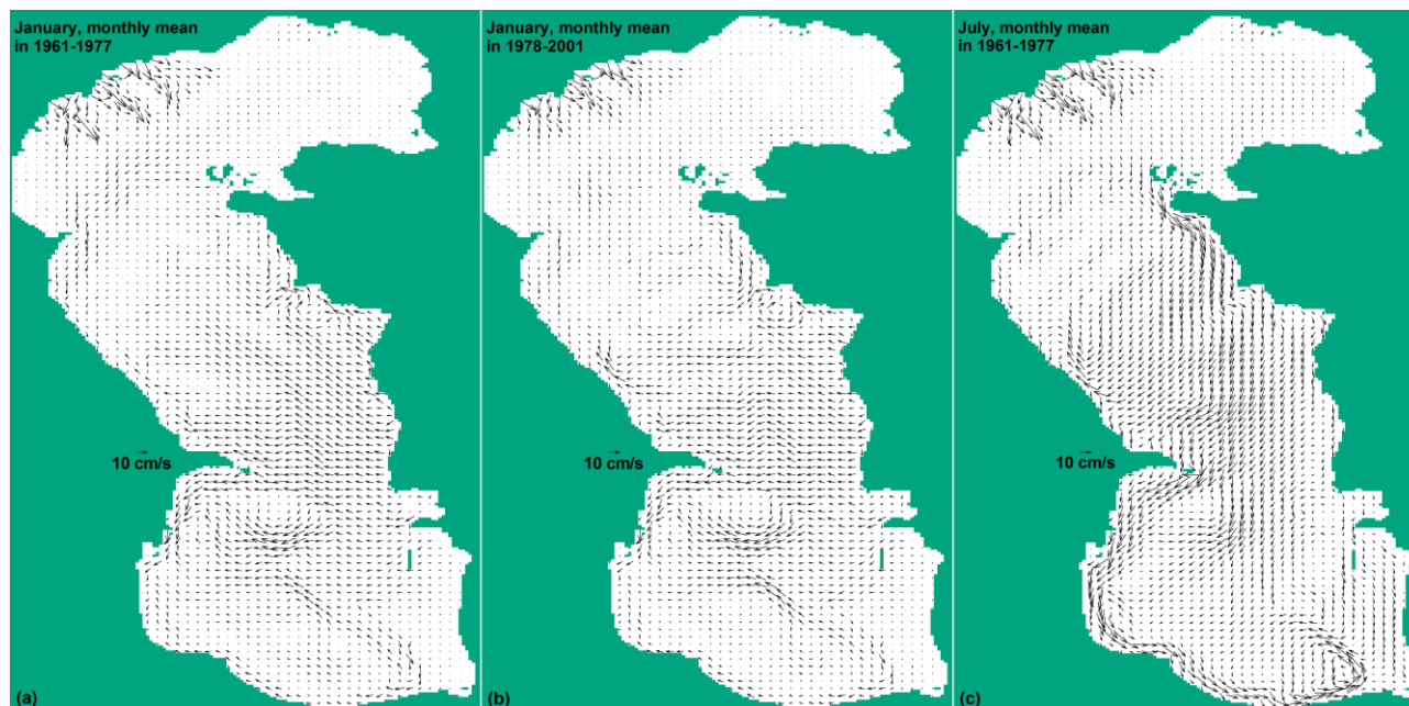
160 Fig. 3. Model monthly mean surface currents in January (a and b) and July (c) averaged over 1961-1977 (a and c) and 1978-2001 (b).
