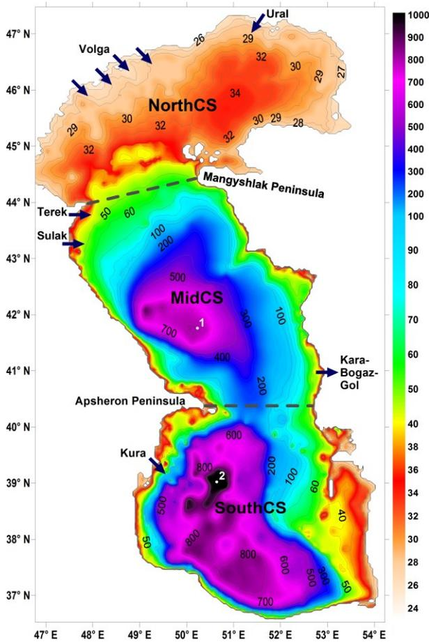
Fig. 1. Caspian Sea bathymetry, used in the model (depths relative MSL, m). The average sea surface ~~depth-height~~ and model vertical grid origin are 28 m. Dashed lines indicate conventional separation of the sea into three basins: **N**orthern (NorthCS), **m**iddle (MidCS) and **S**outhern Caspian (SouthCS). Arrows designate water inflows due to rivers accounted in the model and
