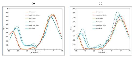
Figure 6. Degree of polarization plotted for the principal plane, i.e., plane containing both incident ray of the sun and zenith direction (cross-section through polar plots for azimuths  $0^{\circ}$  and  $180^{\circ}$ ). Azimuth  $0^{\circ}$  is marked by negative zenith angles. Simulation results for wind speed of 5 m/s for all types of water and two seasons: a) 440 nm, and b) 555 nm.
