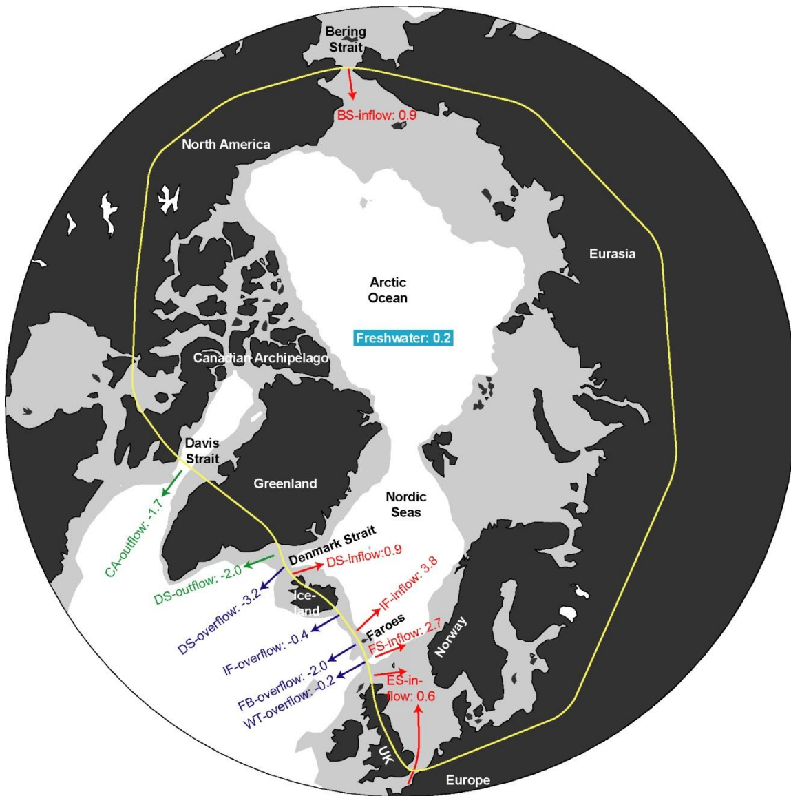
Figure 1. The Arctic Mediterranean (roughly represented by the oceanic areas within the yellow curve) and its exchanges with the rest of the World Ocean. Land areas are black. Ocean areas shallower than 1000 m are light grey. Red arrows indicate inflow branches. Dark blue arrows indicate overflow branches. Green arrows indicate surface outflow branches. Labels for arrows refer to Sect. 2 with numbers indicating average volume transport in Sv ( 1 \text{ Sv} = 10^6 \text{ m}^3 \text{ s}^{-1} ) based on Table 1.
