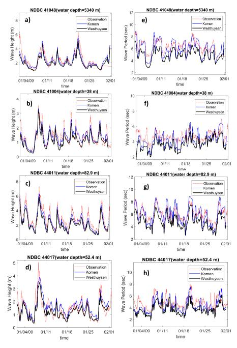
Figure 4: a-d) Time series of simulated wave heights and e-h) simulated mean wave periods, using Komen (blue lines) and Westhuysen (black lines) whitecapping formulas compared to measurements at the four NDBC buoys (dashed red lines).
