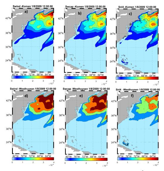
Figure 9: Spatial variations of source terms (wind input, whitecapping dissipation, and quadruplet in  $w/m^2$ ) over the modeling area at time t1, for a-c) Komen and d-f) Westhuysen.
