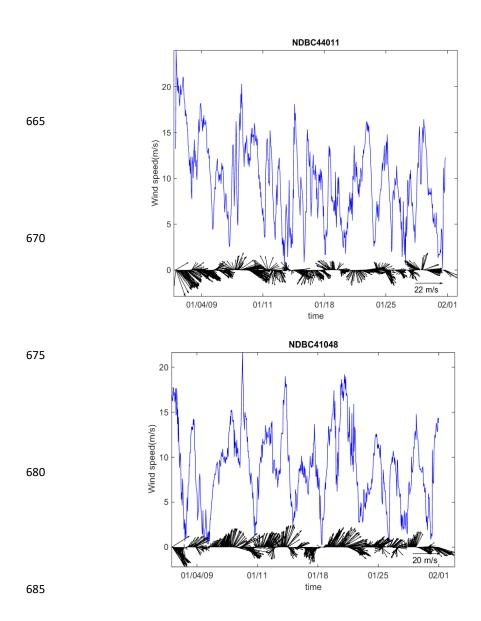
$Figure 2: Time\ series\ of\ measured\ wind\ speed\ (lines)\ and\ vectors\ (arrows)\ at\ NDBC\ buoys\ 44011\ (upper)\ and\ 41048\ (lower).$
