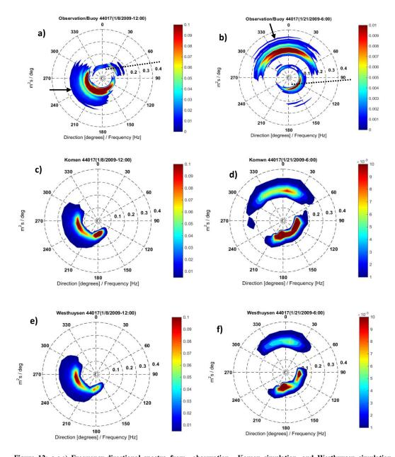
Figure 12: a,c,e) Frequency-directional spectra from observation, Komen simulation, and Westhuysen simulation, respectively at 44017 for time t1, b, d, f) the same spectra at t2. The solid arrows show the direction of observed CFSR wind at the buoy. The direction of the shoreline in the vicinity of the buoy is shown with dotted lines.
