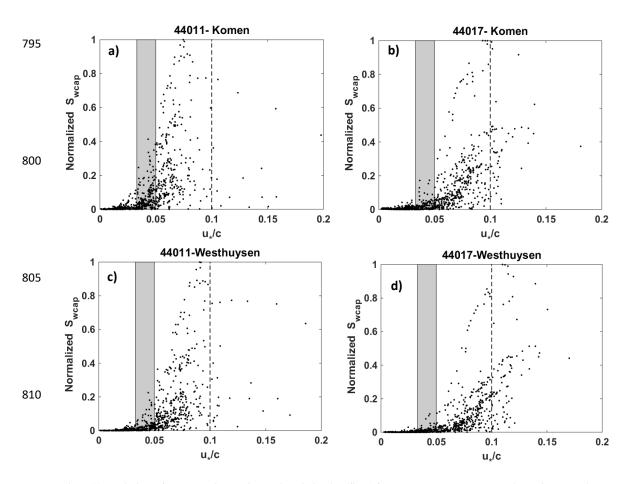
Figure 11: Variations of the normalized whitecapping dissipation ( $S_{weap}$ ) from Komen and Westhuysen simulation scenarios with the inverse wave age  $\frac{u_c}{c}$  at a) and c) NDBC 44011, and b) and d) NDBC 44017. Gray boxes indicate the fully-developed zone (0.033 <  $\frac{u_c}{c}$  < 0.05). The dashed line separates zones for linear and quadratic growth based on Yan(198y) as indicated by  $\frac{u_c}{c}$  = 0.1.
