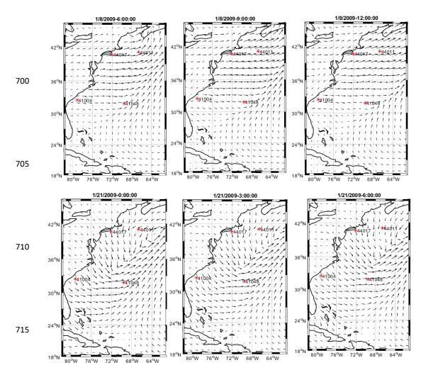
Figure 3: Three-hourly snapshots of CFSR wind fields over the modeling area ending at times t1 (1/8/2009 12:00, upper panels) and t2 (1/21/2009 06:00, lower panels).
