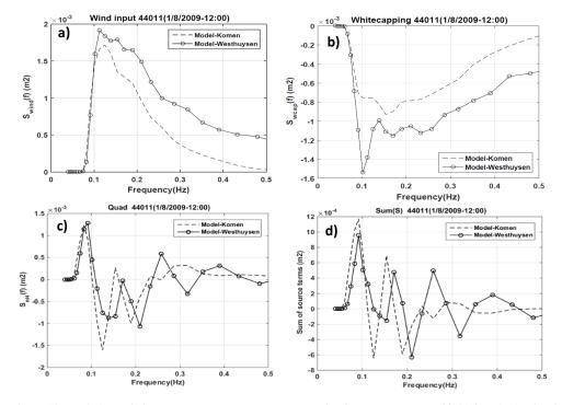
Figure 10: Variations of simulated source term components with frequency at buoy 44011 for t1: a) wind input, b) whitecapping dissipation, c) quadruplet, and d) algebraic sum of these terms.
