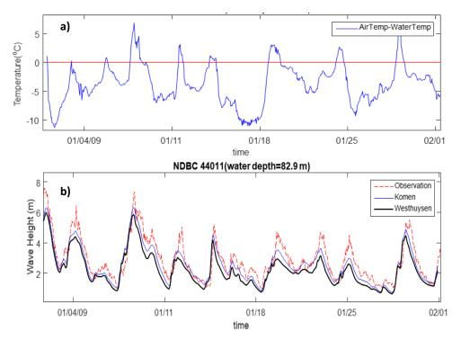
Figure 13: a) Time variations of the observed temperature difference between air and sea surface during January 2009 at buoy 41011. b) Time series of observed and simulated wave heights during this period.
