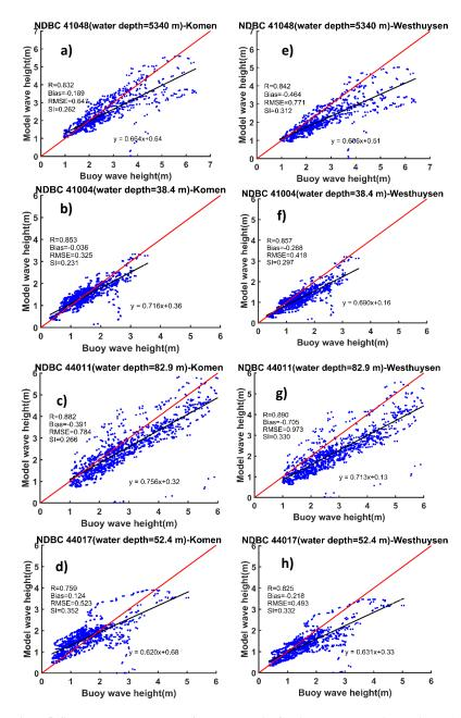
Figure 5: Scatter plots and model performance metrics for simulated wave heights using a-d) Komen whitecapping, and e-h) Westhuysen whitecapping at the NDBC buoys.
