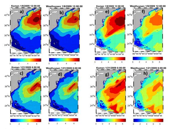
Figure7: a-d) Simulated wave height and direction over the modeling area using Komen and Westhuysen whitecapping formula for timesteps t1 (a and b) and t2 (c and d). e-h) Simulation results for mean wave periods for timesteps t1 (e and f) and t2 (g and h).
