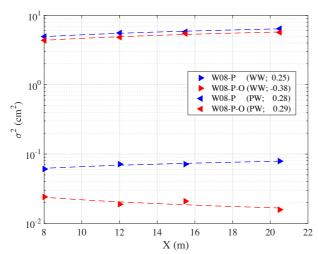
Figure 13: Spatial evolution of the water surface elevation variance  $\sigma^2$  of co-existing wind (WW) and paddle (PW) waves in clean water (W08-P) and with oil slick (W08-P-O). The solid and dashed lines show the power law-type function fitting the experimental data. In the legend the coefficient  $\beta$  of the fitted power law is shown.
