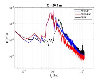
Figure 10: Variance density spectrum  $E(f_i)$  of the water surface elevation z(t) at fetch X = 20.5 m (wave probe G4) in presence of coexisting wind and paddle waves in clean water (W08-P), wind and paddle waves in water with oil (W08-P-O), and wind waves only in clean water (W08). The dashed gray vertical line shows the maximum frequency (2 Hz) produced by the paddle.
