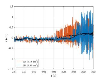
Figure 8: Sea surface elevation at probes G3 (X = 15.5 m) and G4 (X = 20.5 m) for an initially slick-covered surface without oil instillation (experiment W06-O-NI). The dashed and solid black lines show the smoothed elevations (moving average of size 5 s) at G3 and G4, respectively. In the legend, the variance of z(t) within the range of 290 s  $\leq t \leq$  300 s is reported.
