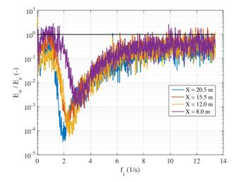
Figure 6: Damping of the wave energy for oil-covered water surface. The damping coefficient is evaluated as the ratio  $D = E_0 / E_c$  between the variance density spectrum of the water surface elevation with oil slick  $(E_0)$  and in clean water  $(E_c)$ . The solid black thin line shows the level  $E_0 = E_c$ .
