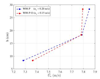
Figure 14: Vertical profile of the wind velocity component Vertical profile of the measured mean horizontal wind speed  $\overline{U}_a$  measured over the water surface at fetch X=11.5 m for co-existing wind- and paddle-generated waves in clean water condition (blue) and for oil-covered surface after the oil instillation (red). In the legend, the value of the friction velocity is shown within brackets. Only the value recorded at the three lowest Pitot tubes are shown.
