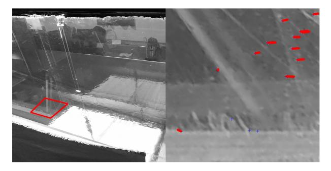
Figure 15: Estimate of surface current speed by optical flow during experiment W06-O. (left) Bounded by a red polygon, the surface
