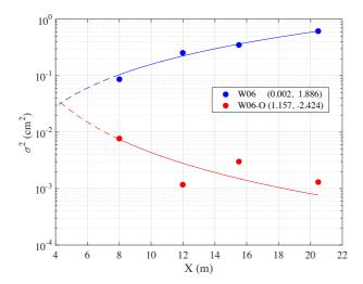
Figure 7: Spatial evolution of the water surface elevation variance  $\sigma^2$  in clean water (W06) and with fish oil slick (W06-O). The solid lines are the power law-type function  $\sigma^2 = \alpha X^{\beta}$  fitting the observations (in the legend, the coefficient  $\alpha$  and  $\beta$ , respectively, are tabulated), while the dashed lines show the laws extended outside the observed data interval.
