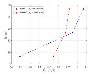
Figure 3: Vertical profile of the mean horizontal wind speed the wind velocity component  $\overline{U}_a$  measured over the water surface at fetch X = 11.5 m. Reference wind speed  $U_r = 6$  m/s. Clean water conditions (blue) and oil-covered surface (red). In the legend, the value of the airflow friction velocity  $u_*$  is shown within brackets. Only the value recorded at the three lowest Pitot tubes are shown.
