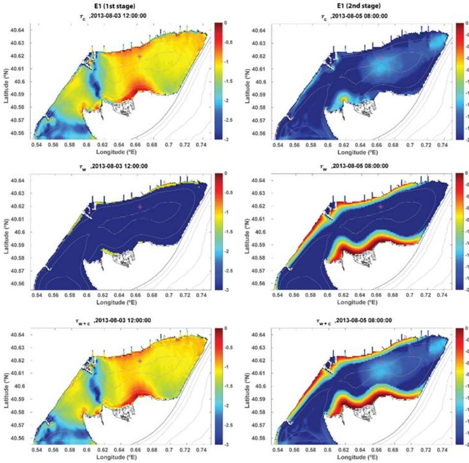
Figure 5: Distribution of the current, wave and combined wave-current bottom stresses  $\log_{10}(\text{Pa})$  in the Alfacs Bay during the first stage of the episode E1 (i.e. seiche; **left panel**) and the second stage of the episode E1 (i.e. sea breeze; **right panel**). Magenta **symbol♦** show the A2 station. Isobaths (in grey) are plotted each 3 m. Note that for clarity, the plot scale is transformed in  $\log_{10}$  and the vertical range differs between both bottom stress distributions.
