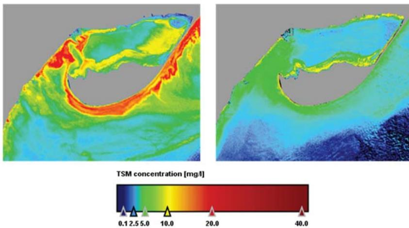
535 Figure 8: Total Suspended Matter (TSM in  $\text{mg}\cdot\text{l}^{-1}$ ) obtained from Sentinel-2 for the Alfacs Bay in two differentiate scenarios: NW winds (left; 27<sup>th</sup> of December 2017) and calm conditions (right; 15<sup>th</sup> of February of 2018).
