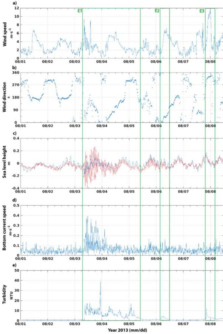
510 Figure 2: Time-series of the variables measured during the field campaign. (a) wind intensity measured in M-Sc. (b) wind direction measured in M-Sc. (c) Sea-level height measured in A2 (blue) and A1 (red). (d) near-bottom current velocity measured in A1. (e) NTU measured in OBS mounted at A2 station. Vertical bars show the episodes considered in the analysis.
