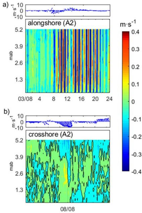
Figure 3: Each panel shows on the top the wind measured at M-Sc (in  $\text{m}\cdot\text{s}^{-1}$ ), and on the bottom the vertical profiles velocities measured at A2 (in  $\text{m}\cdot\text{s}^{-1}$ ; mab mean meters above the bottom). In each panel, different events are showed: 32013/8/32013 for alongshore velocities (panel a) and 2013/8/2013 for crossshore (panel b). Black lines show 0 velocity isolines.
