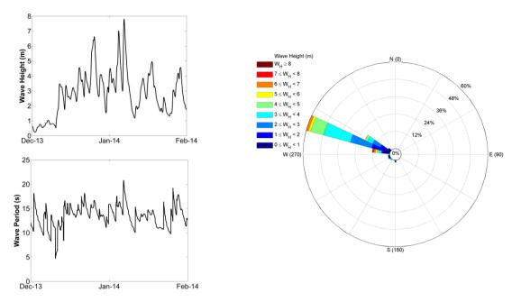
Figure 1 - Wave conditions for the winter of 2013/2014 obtained from the Portuguese Coast wave model in the location of the Port of Lisbon wave buoy.
