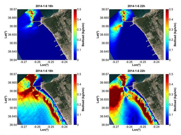
Figure 5 – Results of bed load sediment transport for the scenarios without waves (above) and under extreme wave conditions (below).
