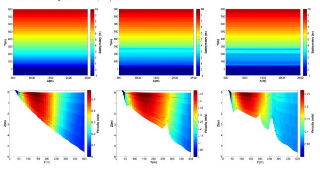
Figure 8 – Simulated sandbars for different wave heights. The horizontal plane of the bathymetry (above) and a vertical cut with velocity modulus and vectors (below). Left: Initial condition. Middle: After 45 days of morphological evolution with 1.5 m wave height. Right: After additional 45 days of morphological evolution with 1.0 m wave height.
