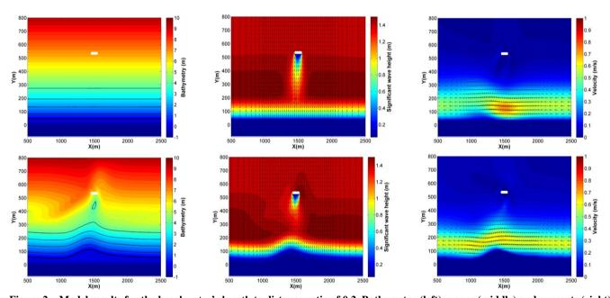
Figure 2 – Model results for the breakwater's length to distance ratio of 0.2. Bathymetry (left), waves (middle) and currents (right) for the initial condition (above) and near equilibrium (below) after 9 years. The thicker isoline in the bathymetry represents the shoreline, whereas the remaining represent the 1 m, 2 m, 3 m and 4 m isobaths.
