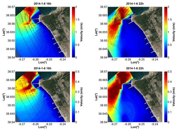
Figure 2 – Velocity results of the Costa da Caparica model during flood (left) and ebb (right) tides at the surface (above) and near the bottom (below) without considering the wave's effect on the hydrodynamics.
