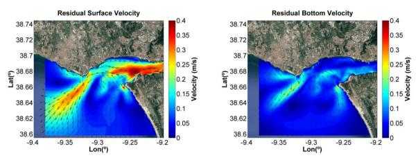
Figure 10 – Residual velocity in the Tagus Estuary mouth at the surface (left) and near the bottom (right) obtained from the three-dimensional baroclinic model for the Tagus Estuary.
