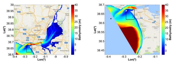
Figure 9 – Bathymetries of the Tagus Estuary hydrodynamic model (left) and the wave model (right) created to propagate the waves until the Tagus Estuary mouth. The domain of the Costa da Caparica model is presented by the black rectangle and the location of the Port of Lisbon wave buoy is indicated by the black triangle.
