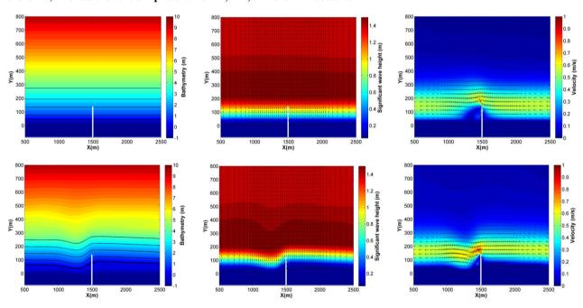
Figure 6 - Groyne with a length of 100 m from the shoreline. Bathymetry (left), waves (middle) and currents (right) for the initial condition (above) and near equilibrium (below) after 9 years. The thicker isoline in the bathymetry represents the shoreline, whereas the others represent the 1 m, 2 m, 3 m and 4 m isobaths.
