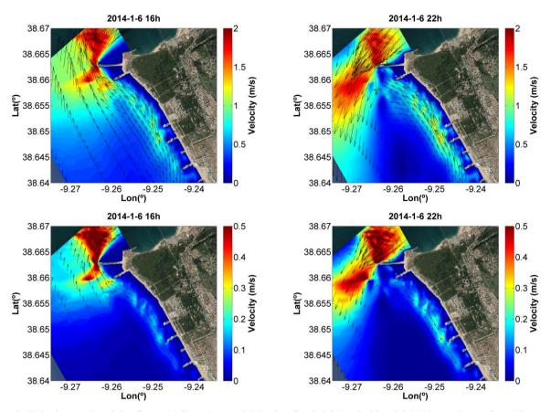
Figure 4 - Velocity results of the Costa da Caparica model during flood (left) and ebb (right) tides at the surface (above) and near the bottom (below) considering the wave's effect on the hydrodynamics.
