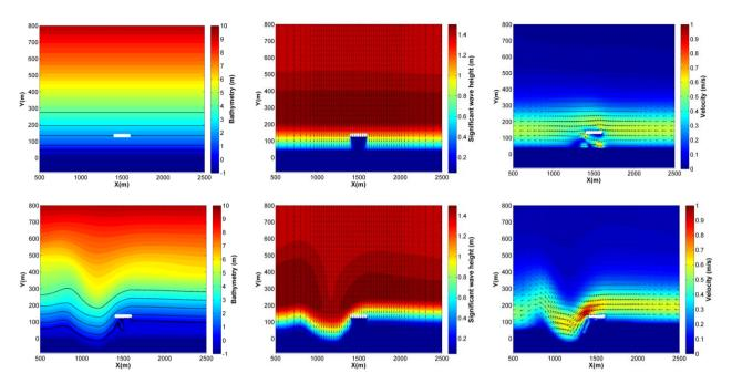
Figure 5 - Model results for the breakwater's length to distance ratio of 2.0. Bathymetry (left), waves (middle) and currents (right) for the initial condition (above) and near equilibrium (below) after 18 years. The thicker isoline in the bathymetry represents the shoreline, whereas the others represent the 1 m, 2 m, 3 m and 4 m isobaths.
