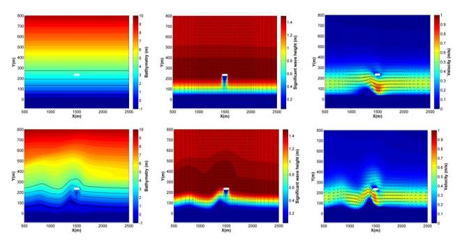
Figure 3 – Model results for the breakwater's length to distance ratio of 0.5. Bathymetry (left), waves (middle) and currents (right) for the initial condition (above) and near equilibrium (below) after 18 years. The thicker isoline in the bathymetry represents the shoreline, whereas the others represent the 1 m, 2 m, 3 m and 4 m isobaths.
