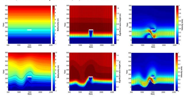
Figure 4 – Model results for the breakwater's length to distance ratio of 1.0. Bathymetry (left), waves (middle) and currents (right) for the initial condition (above) and near equilibrium (below) after 27 years. The thicker isoline in the bathymetry represents the shoreline, whereas the others represent the 1 m, 2 m, 3 m and 4 m isobaths.
