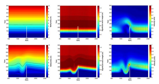
Figure 7 – Groyne with a length of 200 m from the shoreline. Bathymetry (left), waves (middle) and currents (right) for the initial condition (above) and near equilibrium (below) after 9 years. The thicker isoline in the bathymetry represents the shoreline, whereas the others represent the 1 m, 2 m, 3 m and 4 m isobaths.
