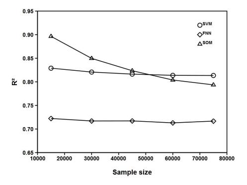
Figure 1: Correlation coefficient between modelled and observed fCO2. The sample size is the number of data points randomly selected to train FFN and SVM and to label SOM.
