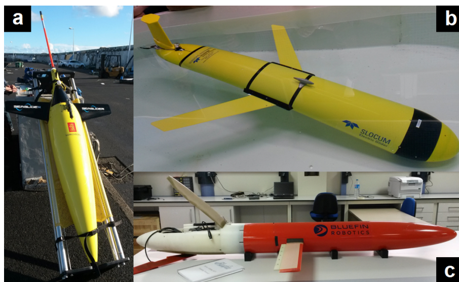
Figure 1. a Seaglider, b Slocum electric glider, and c Spray glider.
