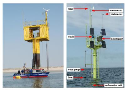
6 Fig. 4. The measuring poles at Spiekeroog and in the inner Hörnum tidal basin.
