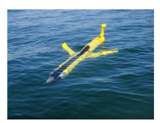
10 Fig. 7. Ocean Glider surfacing to submit data to shore. The glider is equipped with CTD,
