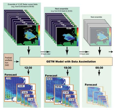
Fig. 161. The functioning of data assimilation and forecasting in the pre-operational COSYNA system. HF radar system covering the German Bight. Radial current components are sent to the HZG data server, where current vectors are calculated and presented on the
