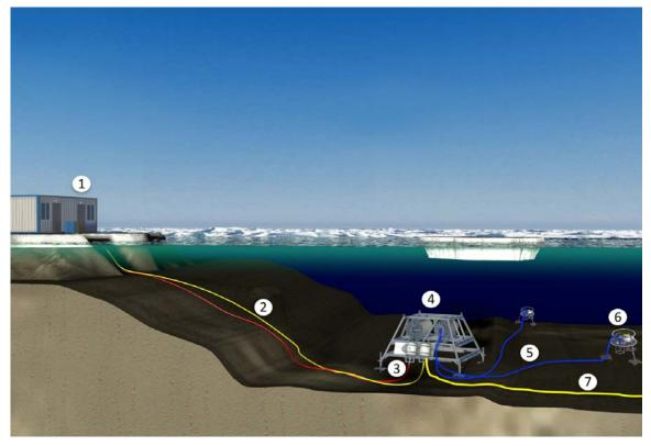
Fig. 81. Setup of the COSYNA Underwater-Node System with (1) land-based server and
