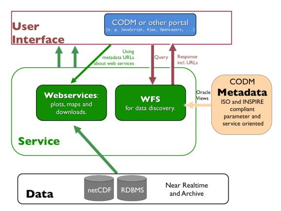
Fig. 25. Data Management architecture: The connection between user interface on one side
