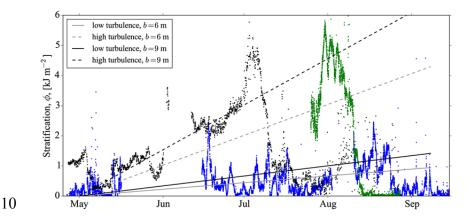
Fig. 7. Measurements showing the observed build up of stratification  $\phi$  over the summer months unaffected by offshore construction (dots; Carpenter et al., 2016) and the estimated rate of stratification removal by the turbine foundation structures in offshore wind farms
