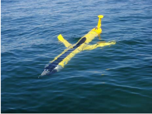
Fig. 7. Ocean Glider surfacing to submit data to shore. The glider is equipped with CTD, optical sensors, and an additional turbulence sensor.
