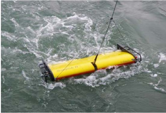
Fig. 20. Scanfish used on regular ship surveys.
