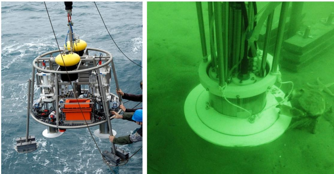
Fig. 114. Left panel: lander FLUXSO deployed for autonomous sampling in June 2015; right panel: sampling chambers in mobile fine sand at 25 m depth.
