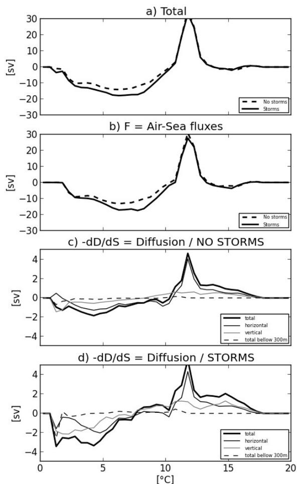
**Fig. 16.** Transformation rate (in Sv) : total (a), contribution of air-sea fluxes (b) and diffuse fluxes across isotherms for the 2-km simulations without storms (c) and with storms (d). The diffuse fluxes are separated into vertical (light gray) and lateral (black) contributions. The dashed lines in (c) and (d) correspond to transformation by diffuses fluxes below 300 m depth. Model transports have been multiplied by 10 in order to scale them to the full Southern Ocean.
