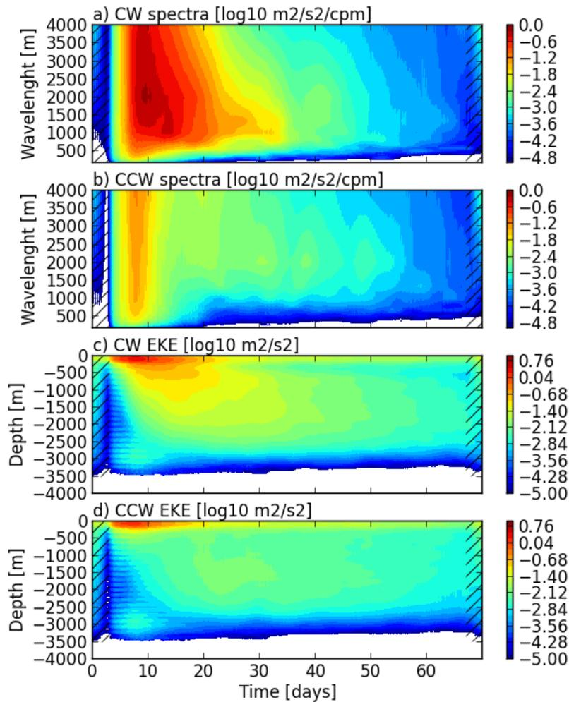
**Fig. 9** : Temporal evolution of clockwise (CW) and counterclockwise (CCW) spectra as a function of vertical wavelength, computed from WKB stretched near inertial velocities (a,b) for the single-storm experiment. Units are  $\text{m}^2 \text{s}^{-2} \text{cpm}^{-1}$ . Near inertial KE computed as a function of time and depth from CW and CCW stretched velocities are shown in (c) and (d). Units are  $\text{m}^2 \text{s}^{-2}$ .
