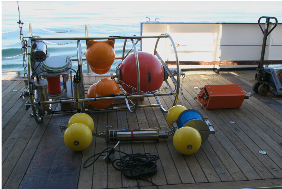
Figure 6. Mooring components laid out on deck before the second deployment in July 2010. Recovery system with acoustic releaser in the front, underwater winch back left and profiling platform with instruments back right.
