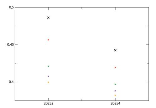
**Fig. 1.** RMS error on temperature (on the whole domain), after the filter analysis (black), and the smoother analyses withÂă: 2 (red), 6 (green), 10 (purple) or 16 (orange) days retrospective assimilation.
