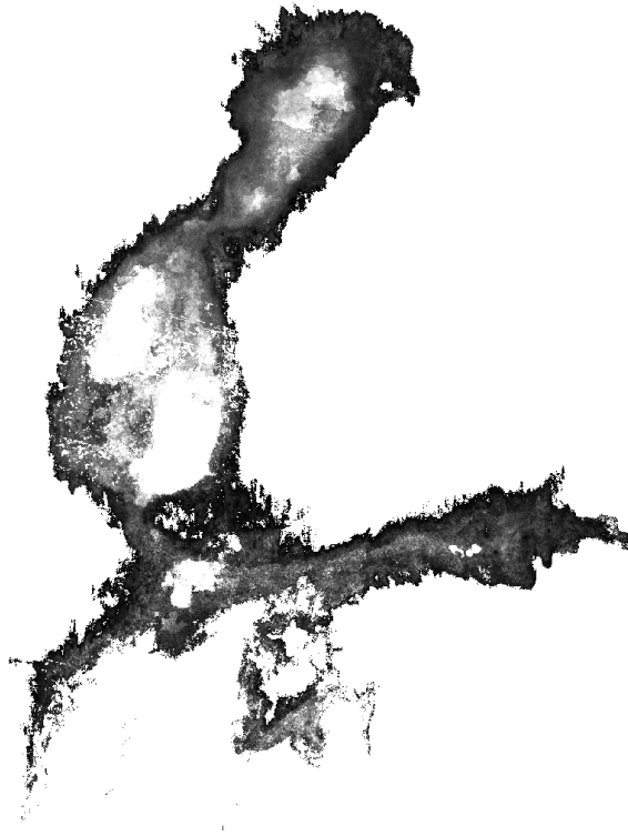
Fig. 5. Mean ice motion magnitude for two weeks before March 5, 2010 based on our SAR ice drift algorithm. Bright tones represent larger motion. The fast ice areas can be derived from this data. The bright areas in the southern parts of the Baltic Sea are open water, open water has been masked off, using the method presented in (Karvonen et al., 2005) and set white in the figure.
