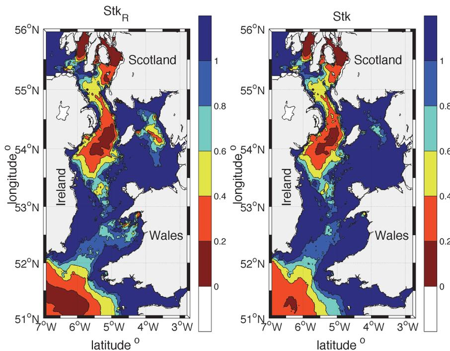
**Fig. 3.** Rotational (a) and non-rotational (b) Stokes number for the Irish Sea.
