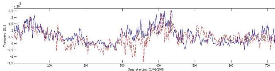
**Fig. 6.** Time-series (2009–2010) of transport in the Corsica Channel. Red dashed line: transport derived from moored current meters. Blue continuous line: transport calculated from ROMS solutions for the same period from the approximately same location.
