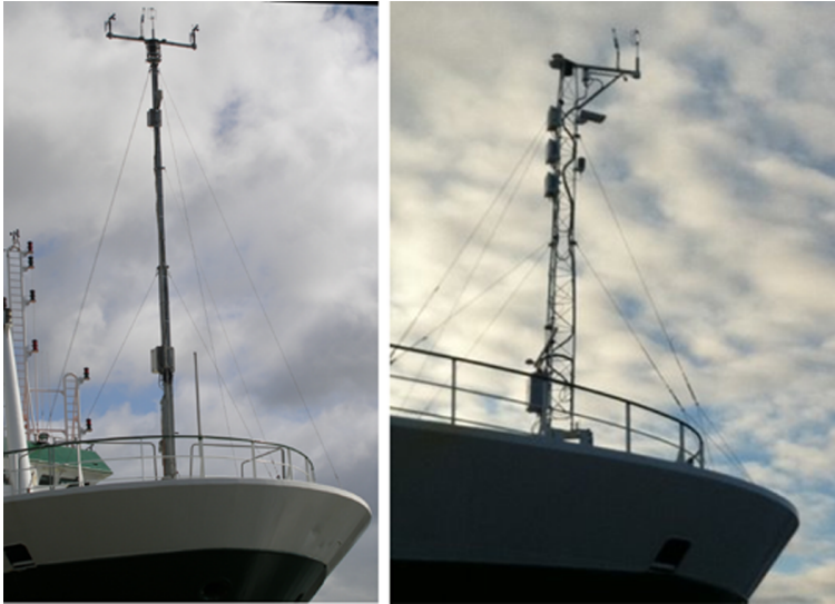
Fig. 2. Photos of the two masts that have been used in this study: left is the single pole mast with a cross beam for the anemometers. Right shows the triangular lattice mast with the sonic located on a boom towards the bow.
