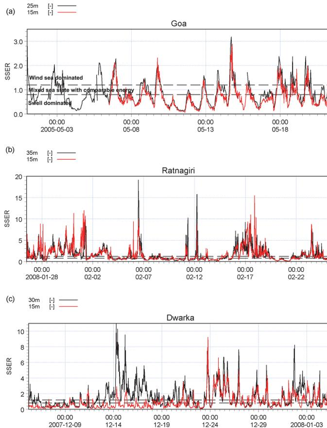
**Fig. 3.** SSER of wind sea, mixed sea and swell: **(a)** 15 m and 25 m depths off Goa, **(b)** 15 m and 35 m depths off Ratnagiri and **(c)** 15 m and 30 m depths off Dwarka.
