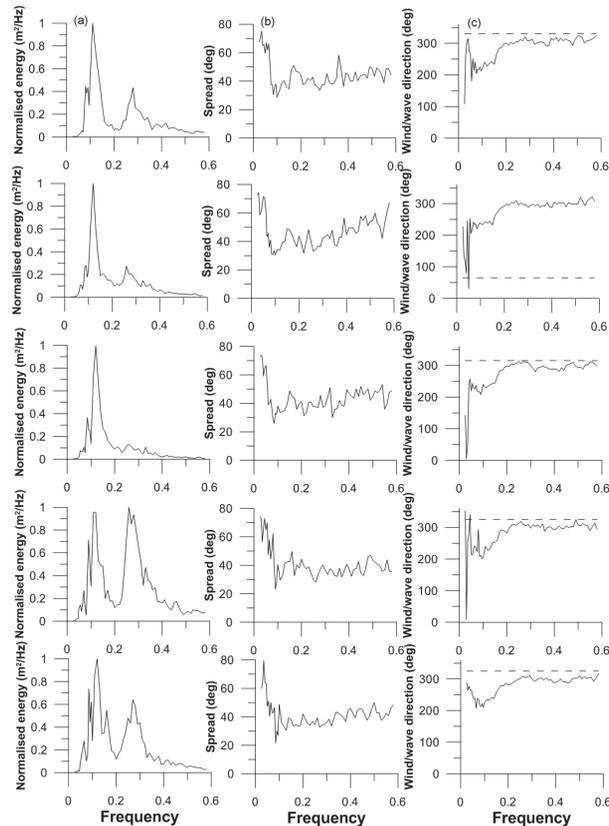
**Fig. 4.** (a) Wave energy spectrum (b) wave spread and (c) mean wave (solid line) and wind (dashed line) directions at 00:00 h, 06:00 h, 12:00 h, 18:00 h and 23:00 h off Goa during 9 May 2005.
