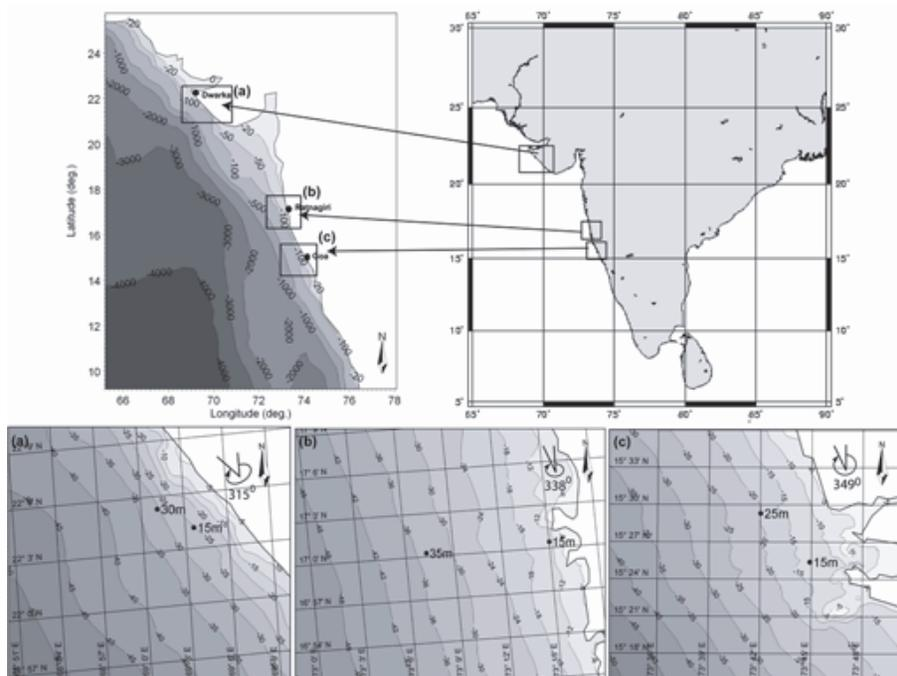
**Fig. 1.** Wave measurement location and its bathymetry contours along the west coast of India. Angles mentioned in the figures are the orientation of the coastline w.r.t north.
