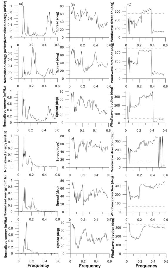
**Fig. 6.** (a) Wave energy spectrum (b) wave spread and (c) mean wave (solid line) and wind (dashed line) directions at 00:00 h, 06:00 h, 11:00 h, 13:00 h, 17:00 h and 23:00 h off Dwarka during 22 December 2007.
