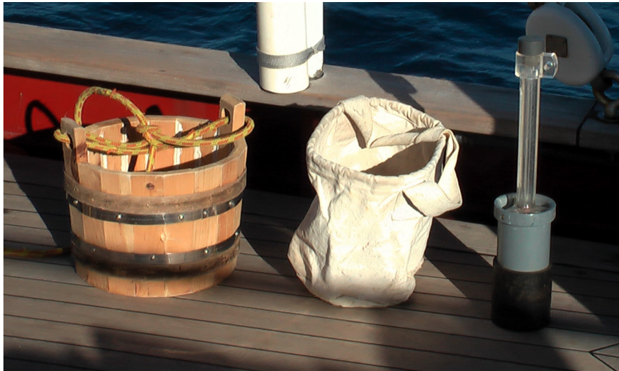
Fig. 2. From left to right; the wood, canvas and rubber buckets used in our field comparison. Note that the wooden bucket was sealed with white caulk along the inner seams and reinforced around the outside by two stainless steel bands. The rubber bucket is of both plastic and rubber construction with a black rubber protective layer around the base.
