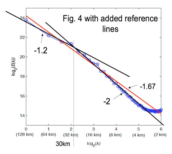
Your fig. 4 with added reference lines, slopes -1.2, -2 (solid black). The dashed line indicates the cross-over point at about 30 km.
